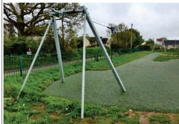
Finding: The surfacing dimensions are short and do not meet with the requirements of the current applicable standard (2.0m required / 1.05m provided)
