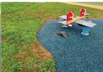
**Action:** Ensure that a suitable impact attenuating surface is established
