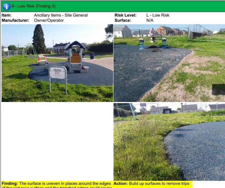
**Finding:** The surface is uneven in places around the edges **Action:** Build up surfaces to remove trips of the wet pour surface and the trenched edges could cause ankle roll injuries
